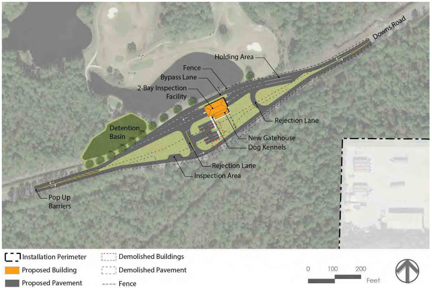
Figure 2.6: Commercial Vehicle Inspection Gate Rendering
